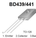
BD439 Collector cut-off current  $T_j = 25\text{ }^\circ\text{C}$   $I_{CEO} < 100\text{ }\mu\text{A}$
