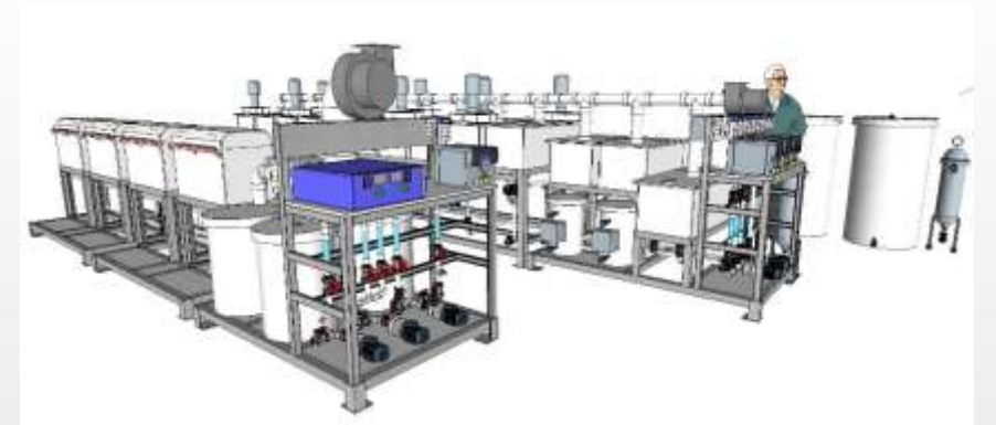
3D model of the solvent extraction facility
